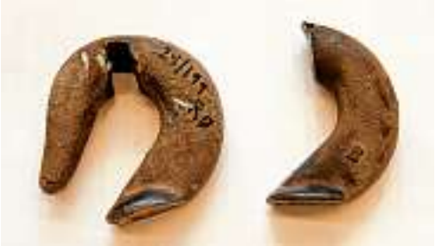
The fire was triggered when a nearly century-old hook snapped, left. The transmission line that failed, known as the Caribou-Palermo, was built in 1921 in the Sierra Nevada mountains, above, by the Great Western Power Co.
