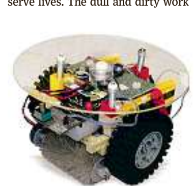
A Roomba predecessor made with Lego, tape and a bottle brush.
