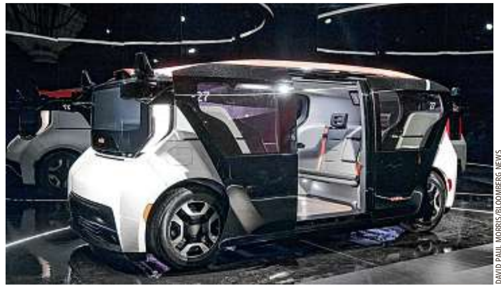
The driverless Cruise Origin shuttle wouldn't have a steering wheel or manual controls.
