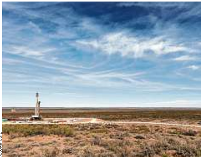
A drilling rig designed for drilling safely near potash mining areas.
