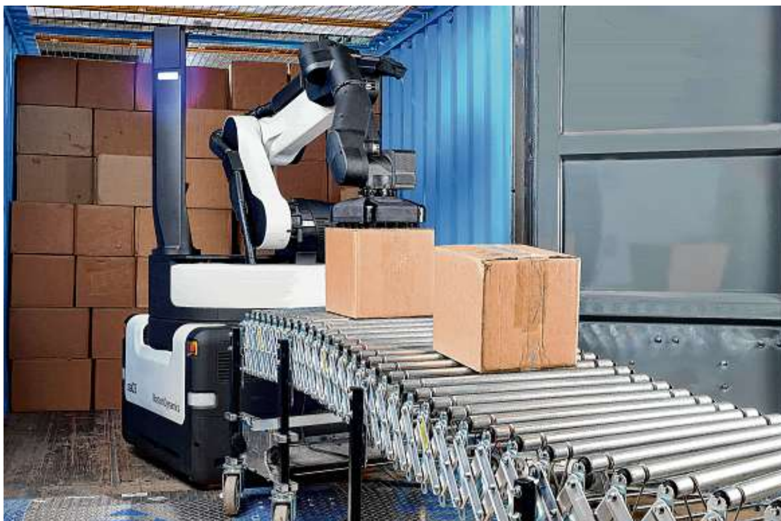
Boston Dynamics' four-wheeled Stretch robot can unload boxes from shipping containers or trucks.
