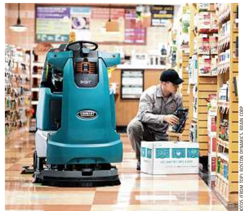
A floor scrubber modified to operate autonomously via Brain Corp. software.
